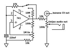
frequencies may vary depending on the 741, you want to test various values and find the ranges you like. Thanks to a slide switch mounted near the PCB's edge, audio or LFO range can be switched easily.
