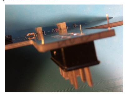
13. Slot the cover along the 4 component legs, snip the exceeding leg and solder the cover.
