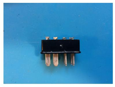
11. Solder the Jones plug. Fill in the holes with solder.
