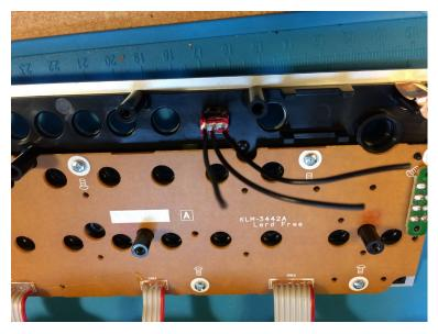
8. Run the cables through the holes of the removed jack socket emplacement, put the sequencer PCB back in place and rescrew it. Screw the standoffs in the panel corner holes.
