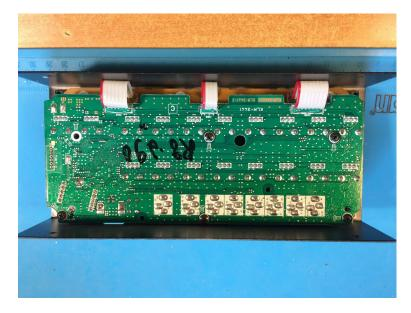
3. Unstick the circuit from the panel using a flat screwdriver, it's sticked with double sided tape and should come easily.
