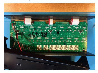
2. Desolder the batteries cables.
