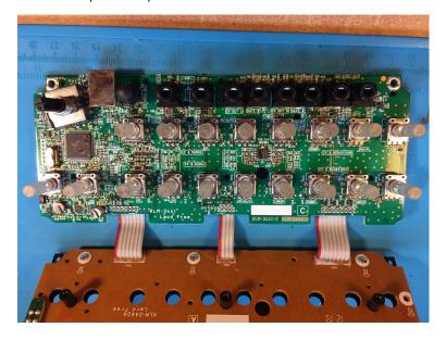
5. Unsolder the first jack socket (littleBits OUT) located to the right of the power pushbutton and enlarge the mounting holes with a hand drill.
