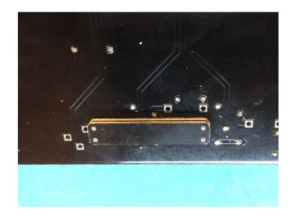
15. Connect the sequencer circuit to the SQ-1 Card. The CV and gate cables to the corresponding jack tips. The 0V cable goes to the closest jack sleeve. The +5V cable to the solder joint shown on the close-up pic. The switch cables to the pads in front of their holes.
