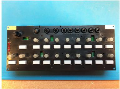
4. Unscrew the 6 PCB black screws and open the sequencer
