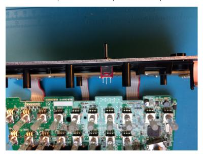
7. Solder 3 cables to the subminiature switch.
