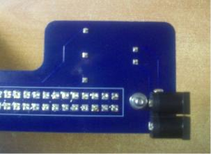
If the optional PSU is not used, bridge the "208 supply" pads to the right to power the Hub's +/-15V rails with the 208's ones, with headers + jumpers or solder components legs.
