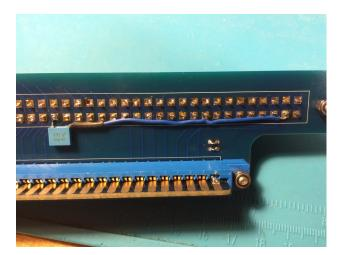
5. Not all edge connectors have the same depth. Depending on your 208's one, bad contacts may occur because the transfer card between the Hub and 208 is not pushed deep enough into the 208's connector. To fix this, insert a piece of wire into the Hub's connector so that the transfer card protrudes a little more. You can solder the transfer card's contacts 1 and 28 to the Hub's edge connector to prevent it from staying in the 208's edge connector when the Hub is unplugged.
