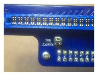
It is still possible to use the 208 supply with the Artesyn AEE00CC18-LS block installed to the Hub as long as it's not powered with an external DC supply.
