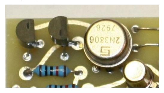
On **board 6 and 7** mount the **pA726** with components leads and avoid pin headers. In many 208s that I repaired bad contacts in headers caused mute or unstable oscillators.
