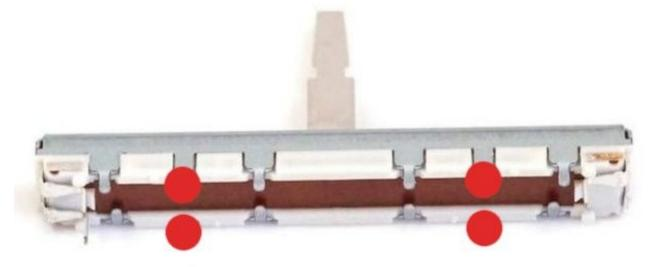
**For the bare tracks revision only:** before mounting the **9mm Alpha snap-in pots** to the motherboard, bend the metal tab under the CO fine tune and waveshape pots to prevent the risk of short with the PCB trace under the pot.
