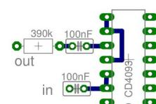
You can also do connections directly to the rear of the edge connector and use the "to prog" sockets of the 208 panel as inputs. These inputs already have resistance, thus you want to slightly lower the value of the resistor you'll use. Here again there's no fixed rule, feel free to experiment and find what best suits your needs. Connect a 180k resistor between front pin 26 and rear pin 28 will give CV input to the LPG2 routing switch on the preamp "to prog" socket.
