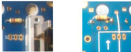
An extra 100nF cap is needed in series with the 390k resistor mounted between the CD4093 and EG looper switch.
