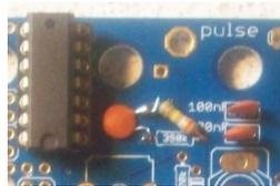
Do not socket the TL072, the socket might upset the adjacent slider's alignment with the panel. Place the TL072 as far as possible from the slider, slightly offset it from the silkscreened drawing and bend its legs (and yes a TL082 can do the job :)).
