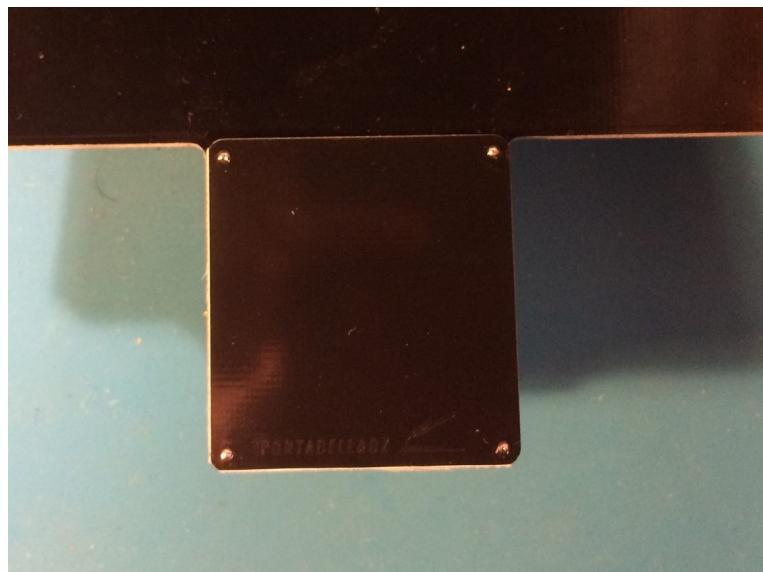
14. Proceed the same way to install the small plates of the handle support to the back of the SQ-1 Card.
