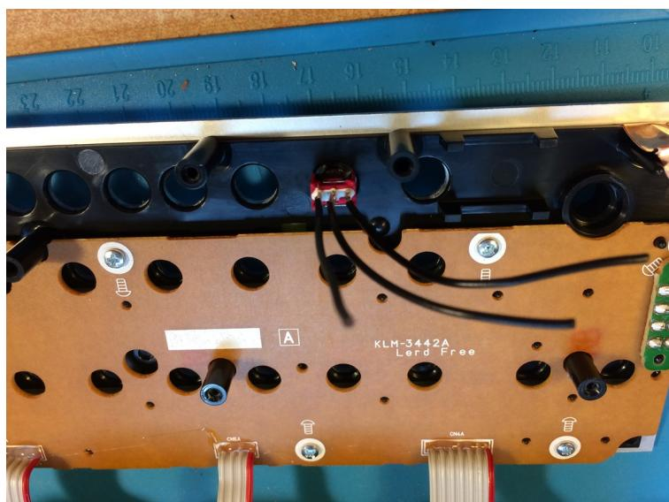
8. Run the cables through the holes of the removed jack socket emplacement, put the sequencer PCB back in place and rescrew it. Screw the standoffs in the panel corner holes.
