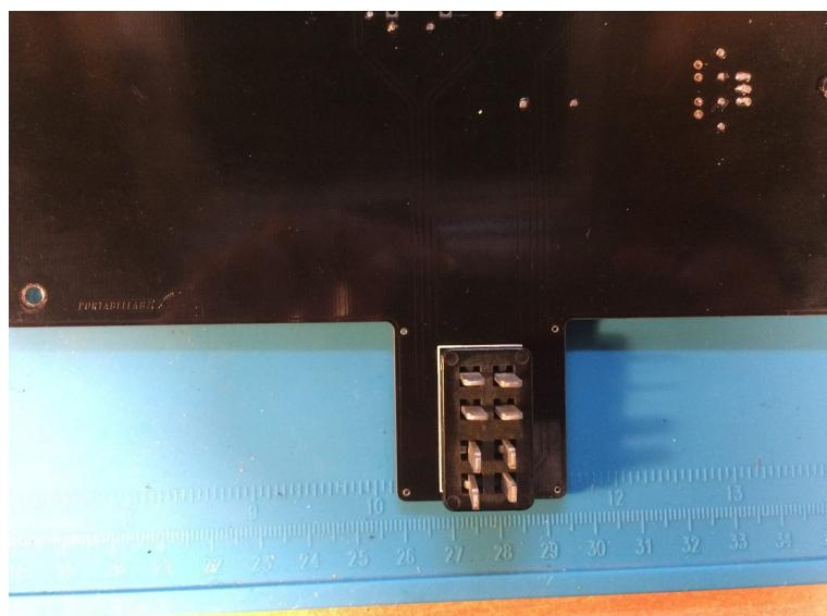
12. Solder a component leg in each of the 4 holes in the corners.
