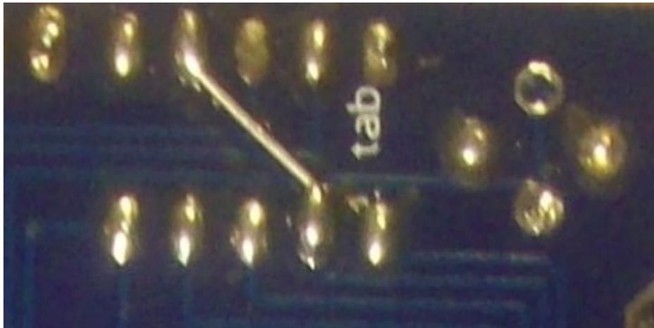
On the new pA726 shipped **after January 20th** (with rounded corners) this bridge is not needed.
